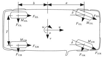
Figure 1 Schematic Vehicle with Seven Freedoms
