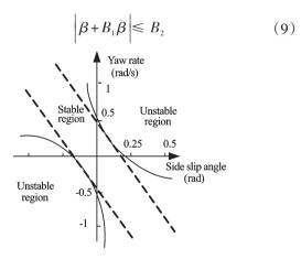
Figure 4 the Stability Rule of Yaw Angle
